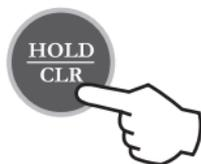
The H symbol blinks to indicate that the display is in hold mode. Press the HOLD key again to return to normal operations.
