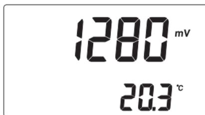
Since mV readings are not temperature compensated, the ATC and MTC tags are turned off .
