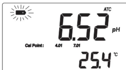
Moreover, when the battery level is too low to ensure reliable readings, the meter automatically turns off. At start-up the display will show “0 bAtt” for a few seconds and then the meter turns off.
