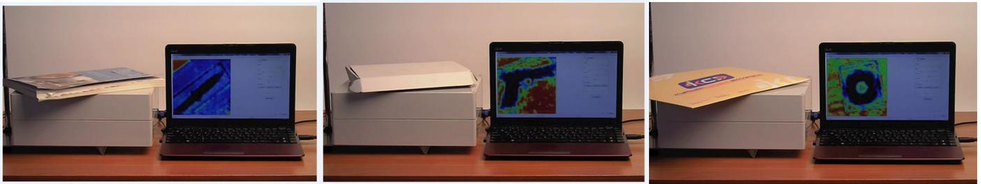
Non-conductive materials, on the contrary, are likely to be fairly transparent. Many types of plastic and rubber, PVC, synthetic foam (polyfoam) some composite materials, wood have fairly low absorption and therefore are transparent in THz light. With some of these materials max thickness (or penetration depth) can reach 10-15 cm. Penetration depth in Teflon, PTFE, Silicon can be higher by an order of magnitude because of their extremely high transmission ratio.
