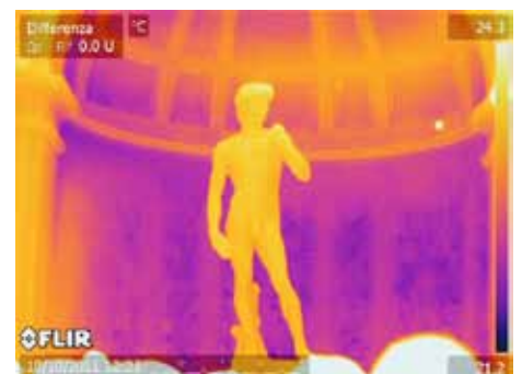
This thermal image reveals the underlying texture of the walls and pillars of the apse in which Michelangelo's David is placed.
