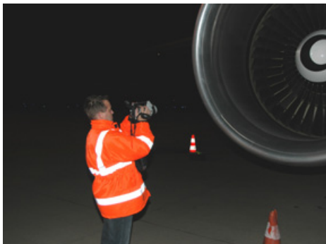
Mr. Ralf Grispen while inspecting an airplane with his FLIR thermal imaging camera.
