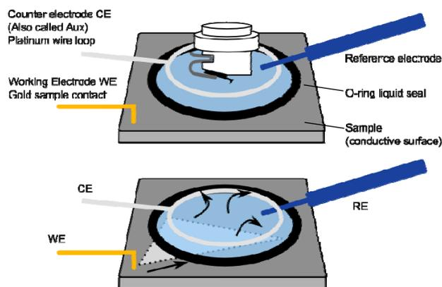
**Fig. 1** Above: the standard 3-electrode system for electrochemistry experiments, as used in the ECCell™. Below: the general current flow. The working electrode is contacted outside the liquid, and surface redox reactions allow the current to flow through the liquid to the counter electrode
