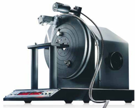
GON 360 for transmission and reflection measurements at variable angles
