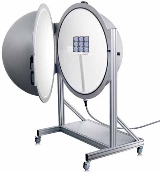
The ISP 1000 integrating sphere with 1 m diameter
