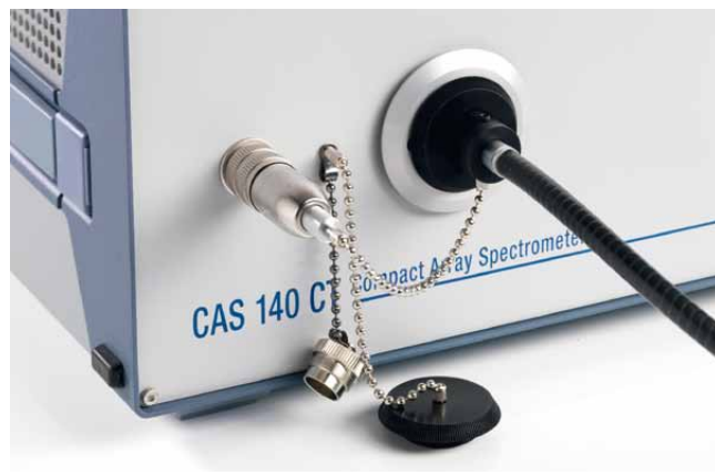
The Ident key identifies measurement adapters
