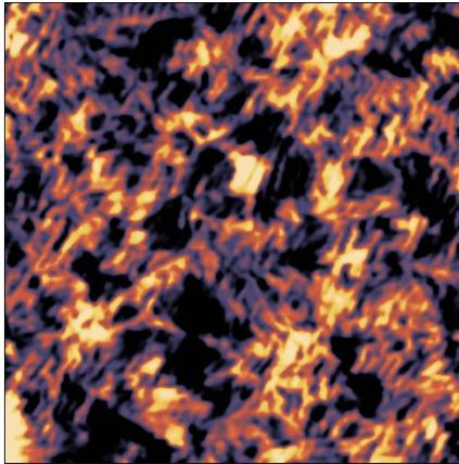
Fig 2: Topography image of crystalline polyethylene (z-range: 15 nm) measured at -120°C, scan size: 2 μm x 2 μm
