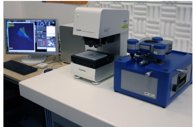
Fig. 1: The JPK NanoWizard® on the BioMAT™ in combination with LEXT OSL4100 from Olympus
