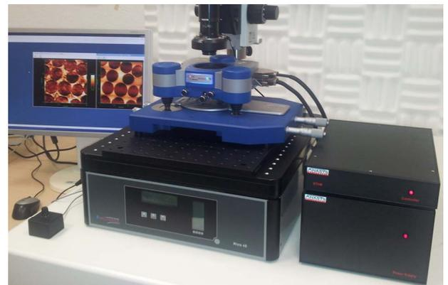
Fig. 1 JPK NanoWizard® 3 AFM and Ansys SThM module
