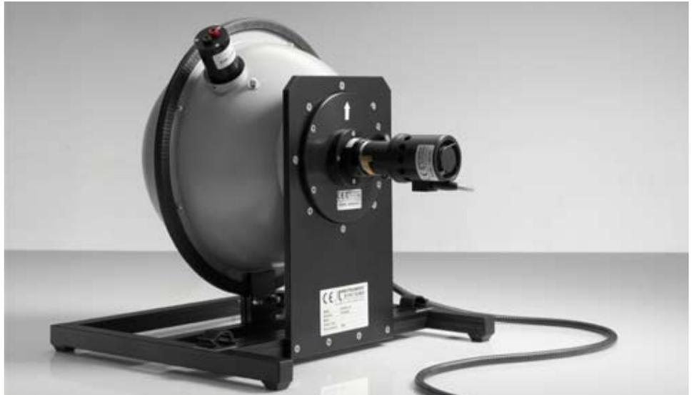
All spectrometers from Instrument Systems can be interfaced with the ISP 250 by means of their fiber-optic connection on the detector port. Special adapter plates and proven LED test sockets are used to mount LEDs and launch the
